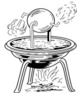
Figure 1.1 Aeolipile of Hero [2]
