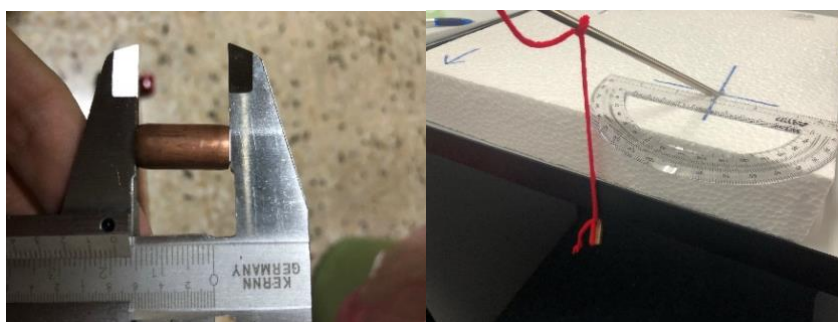
Figure 2. Measurement of mock bullet cartridge (left) and bullet trajectory analysis (right).
